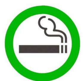
2. The size of the informative symbol may be proportionately enlarged or reduced, however, the external diameter of the symbol shall be not less than 60 mm.
